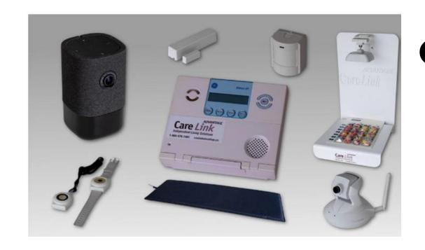
CareLink Advantage is a wearable or non-wearable remote monitoring system that can be customized to deliver services which best meet the needs of the user. This can include motion, door, bed, and motion activated camera.
